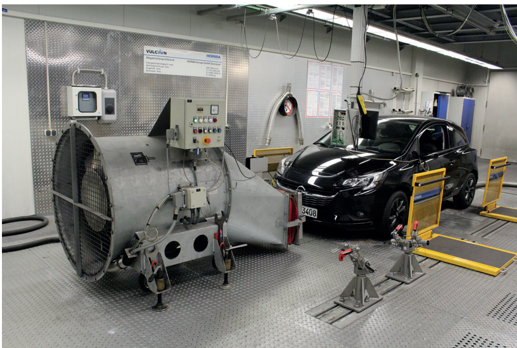
Figure 2: Roller dynamometer test bench used in the measurement of exhaust emissions and fuel consumption
